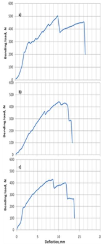
Fig 1. Bending load Vs deflection of a) sinusoidal b) Square and c) triangle core corrugated sandwich with 0.5 mm thick corrugation under three point bending.
