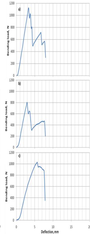
Fig 3. Bending load Vs deflection of a) sinusoidal b) Square and c) triangle core corrugated sandwich with 1 mm thick corrugation under three point bending.
